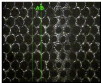
Score lines appear as shiny rings across the circumference of the Anilox roll surface. At high magnification we can see these lines are actually worn areas of cells. This wear is mainly caused by particles of steel that are worn or chipped from the doctor blades. These metal particles become lodged between the doctor blade and the Anilox subsequently destroying rows of cells.
