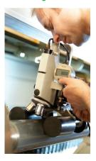
If you are unsure of the condition of one or various of your Anilox rollers and cannot afford to send the anilox off site for a full inspection, you can request Cheshire Anilox Technology to send you a self-diagnostic screen test kit.
