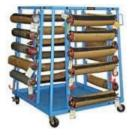
Before storing a roll, the face and journals should be cleaned. The face should be dry and some form of protective cover should be applied. Anilox covers will be the most adequate means to provide great impact resistance while the Anilox is stored. After the face is covered, a lightweight lubricant such as WD 40 should be applied with a rag to the journals. This will reduce rusting and corrosion.
